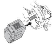
• Press on the lower part of the battery and push it in as far as it will go into the battery compartment. Make sure the latches snap in place properly.
